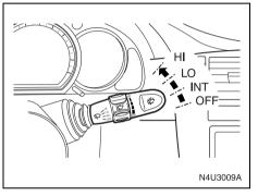
Use the windshield wiper/washer lever to operate the windshield wipers.
